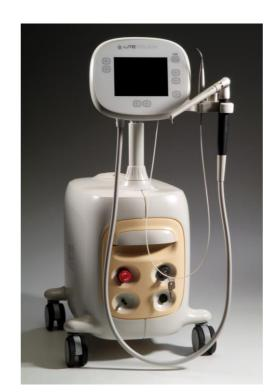
Laser Type: Erbium YAG **Wavelength:** 2.94 microns Pulse Energy: Up to 700 mJ **Pulse Rate:** Up to 50 Hz Pulse Duration: Hard tissue mode: < 0.6 ms Soft tissue mode: < 1.0 ms **Power:** Up to 8 Watts on tissue Spot Size Hard tissue mode: 0.6 - 1.0 mm
